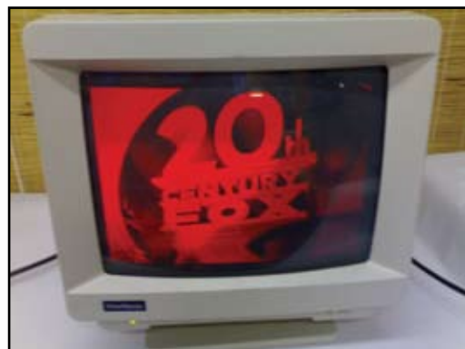
Damaged display cables can create a prominent colour tint
